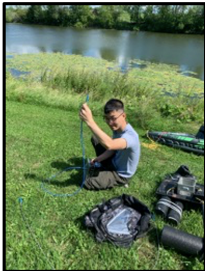
Left image: Measuring the sun's irradiance (light incident on the water surface from above) to set up the optimal integration time of a spectrometer.
